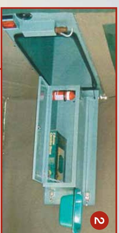
1 Queen bed with gas strutted base allows access to below storage in trailer. Zipped draft skirt allows access to front and rear side toolbox storage 2 Rear swing-out tailgate with built in Mess Locker & pullout basin surround (inbuilt stove option available) 3 Toolboxes and Doors auto dust sealed, lockable and keyed alike
